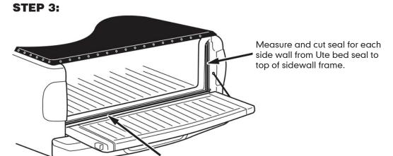
Measure rear face of Ute bed bottom and cut Tailgate seal to fit from sidewall to sidewall. Remove release strip from adhesive tape and apply seal, starting at one end. **DO NOT STRETCH SEAL WHEN APPLYING.**
