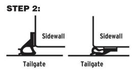
Seal may be installed either along the rear face or the inside surface depening on the tailgate sidewall structure. Cut a small sample and test fit, making sure that bulb end compresses when the tailgate is closed.
